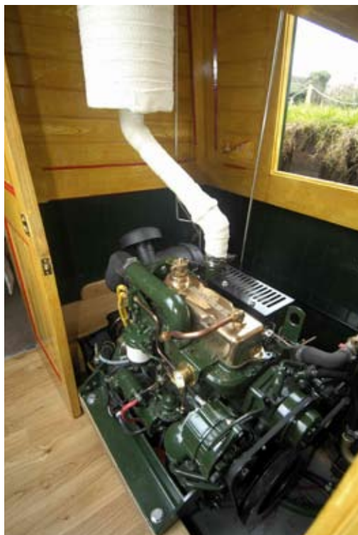
below Beta JD3 Tug engine with emulsion painted exhaust lagging.
